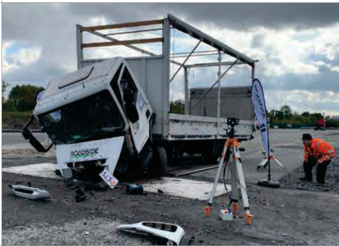
Pictured: Test vehicle after collision with RAM48 bollard.
