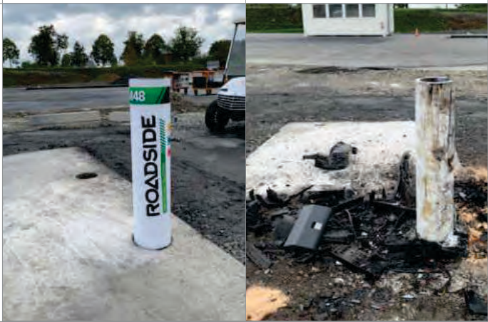
RAM48 bollard before and after impact by test vehicle.
